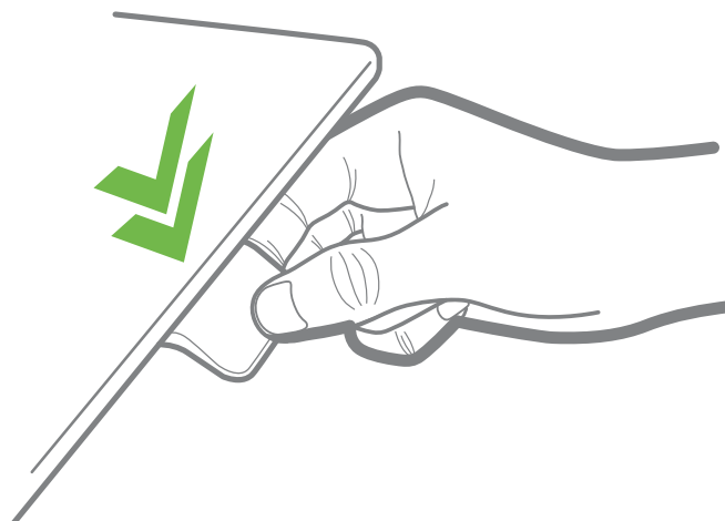
Figure 6 Double-tap the DPI to drive the desk to a pre-set favourite position
